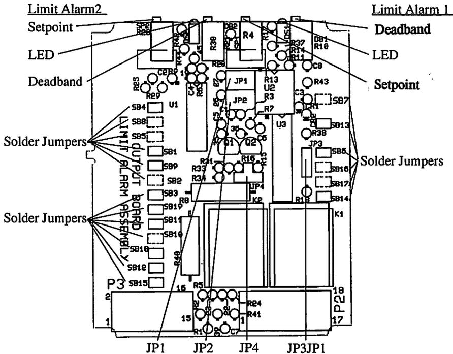
**Series 8000 Dual Limit Alarm Output Specifications**
