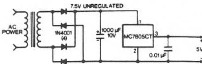
Figure 1. Typical Power Supply
