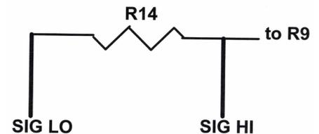
Figure 4. Current Shunt Location
