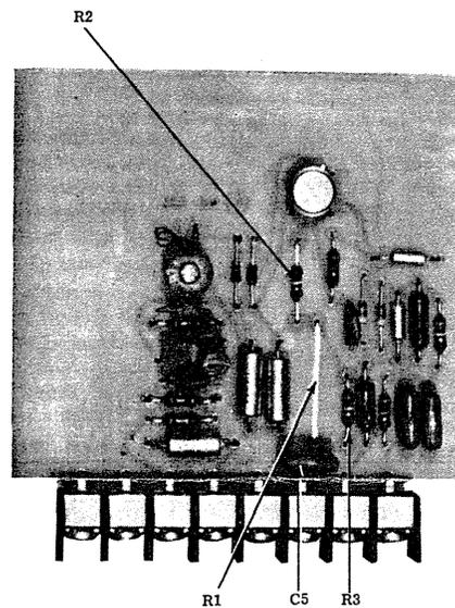
Figure 5. Component Location Upper Board Assembly
