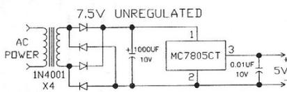
Figure 1: Power Supply Schematic
