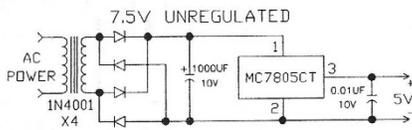
Figure 1: Power Supply Schematic
