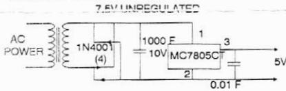
Figure 1. Typical Power Supply Schematic Diagram
